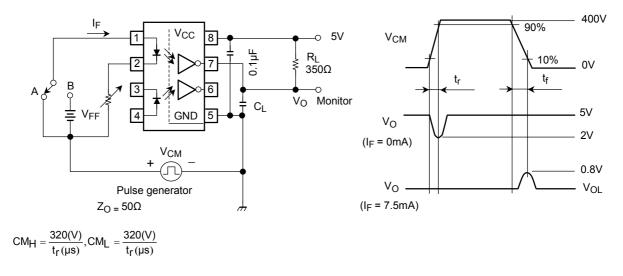
\* C<sub>L</sub> is approximately 15pF which includes probe and stray wiring capacitance.
